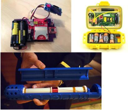
**Figure 3.** Examples of sensor hardware: Noise monitor<sup>59</sup> (left), SweetSense<sup>™</sup> <sup>60</sup> (right), and HealthyShrimp<sup>40,41,61</sup> (bottom).
