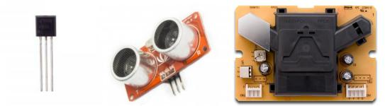
**Figure 2.** Examples of sensing devices (left to right): Parallax temperature<sup>56</sup>, Arduino distance meter<sup>57</sup>, and Shinyei particle sensor<sup>58</sup> (air pollution).
